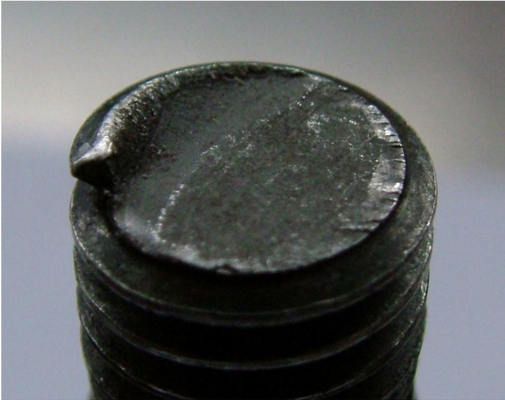
It is easy to see how the initial fracture has started at the base of the thread.
