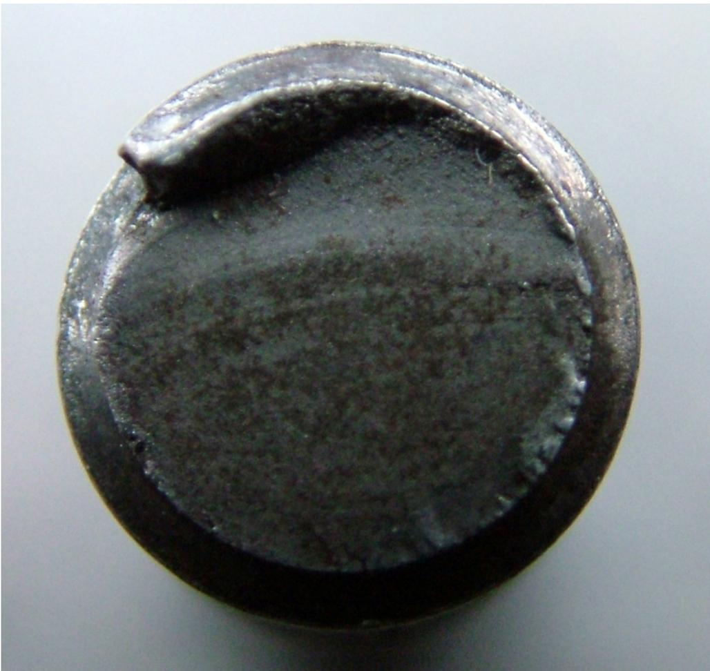
The growth rings are very evident. The fracture has progressed through the bolt until the stress area has reduced to such a small size the bolt has failed under tension.
