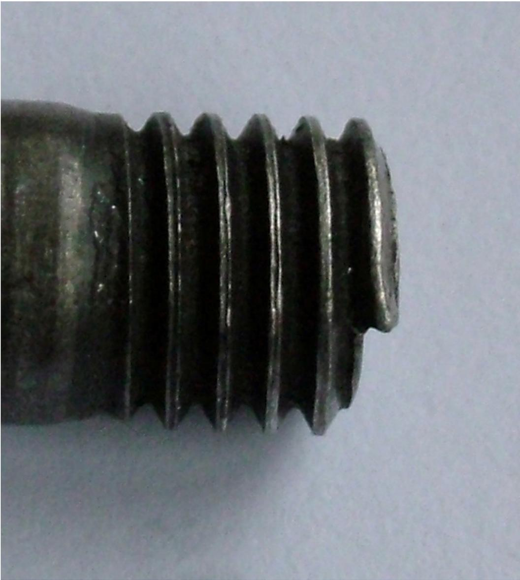
The fact that the thread is bent in the direction of axial load is evidence the bolt ultimately failed under tension.
